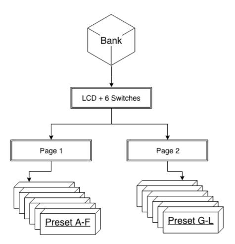
Each bank can display up to 6 presets, of which all are accessible from the 6 switches. The other 6 presets can be engaged via dual switch presses or external aux controllers. A Page Toggle function is also available to switch between the first 6 presets and the last 6 presets.
